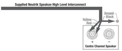
• If connecting a REL as a dedicated rear channel sub, connect the yellow wire to the left rear positive speaker terminal; connect the red wire to the right rear positive speaker terminal, connect the black wire to a ground lug or chassis screw. If the amplifier is of balanced differential design, please follow the instructions in the section above labeled Differential Connection.
