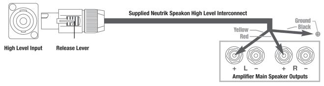
• For Differential(i.e. fully balanced) amplifiers using one REL, simply use the standard connecting scheme above. Connect the black wire to a ground lug or chassis screw. Should hum occur using this method, the black wire should be allowed to "float" or hang down without connection to ANY terminal.
